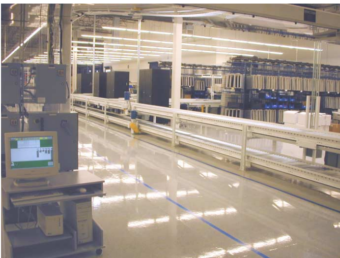
Final assembly highway with Think & Do control PC (left)
