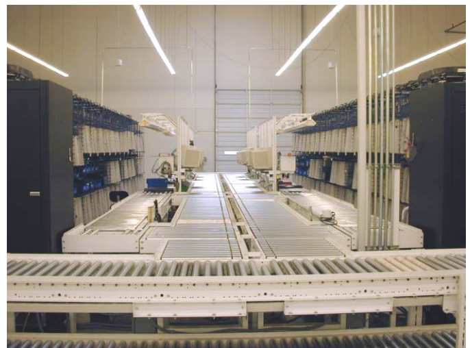
Final assembly spur conveyors
