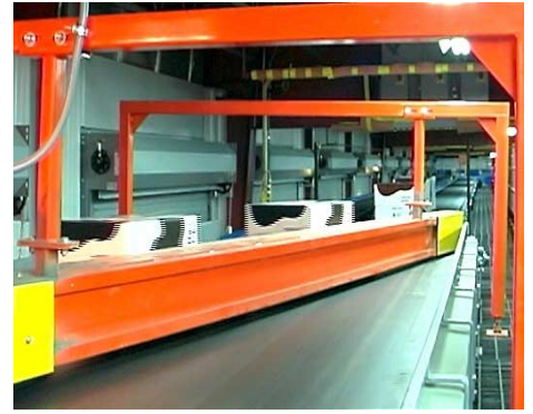
PC cartons move by at a blur on the 375 ft.-per-minute conveyor
