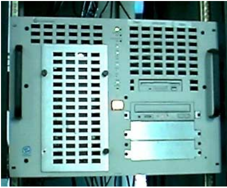
The main auto-sort controller — a Gateway rack-mount server running Think & Do software
