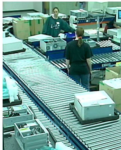
Conveyor delivers nearly-assembled PCs to lidding area
