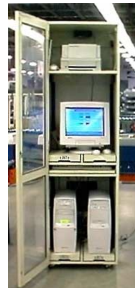
Gateway-designed control cabinet housing lidding conveyor controller
